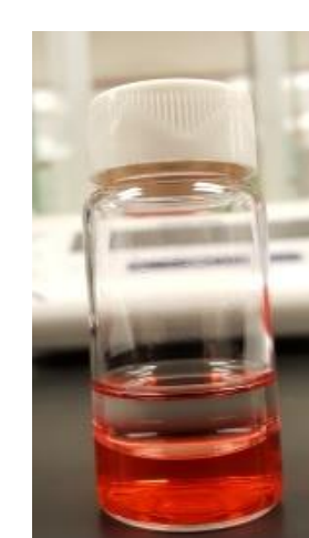
Figure 5 (left): An example of a solvent system for a liquid-liquid extraction. The top organic layer is kerosene, while the bottom layer (shown in red) is an aqueous buffer with pH = 4. As shown in the figure, a sharp boundary separates the two phases.
